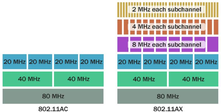
OFDMA divides up the 20 MHz channel into 256 subcarriers. The smallest unit is 26 subcarriers in 2 Mhz of frequency. These subcarriers can be grouped together into larger units; at 52 (4 Mhz), 106 (8 Mhz), and 242 (20 Mhz) to support higher bandwidth applications. Each grouping of subcarriers are called a resource unit (RU).
