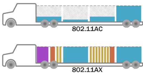
Thus far, the discussion has been limited to a 20 Mhz wide channel. 802.11ax uses OFDMA to subdivide 40, 80, and 160 Mhz wide channels into an increasingly dense number of subcarriers. Additionally, the access point will synchronize upstream OFDMA transmissions from the client to the access point. Thus OFDMA allows simultaneous, multiple client transmissions in each direction.
