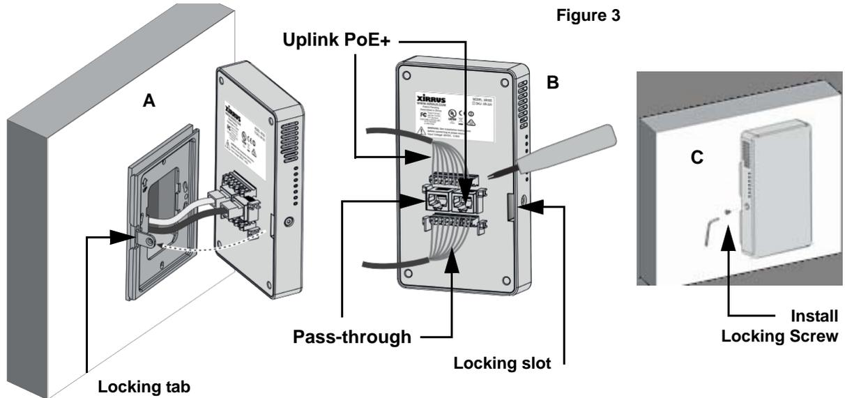
4. Move the AP into position against the bracket. Make sure that the locking tab mates with the locking slot as indicated by the dotted line in Figure 3 (A). Secure the AP to the mounting bracket using the locking screw, as shown in Figure 3 (C). The screw should be tightened to not more than 20Kgf and care should be taken not to damage the equipment.
