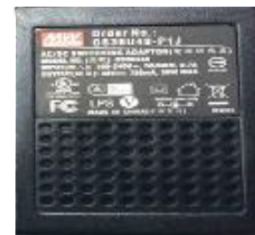
Reference XR-320 External Power Supply: Mean Well GS36U48-P1J
