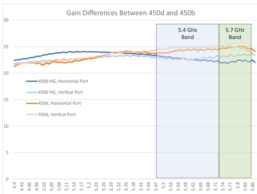
As noted in the graph, the 450b ranges between 1 and 3 dBi lower in gain throughout both the 5.4 and 5.7 GHz frequency bands. The peak gain for the 450b High Gain dish is accurately specified at 24 dBi, while the 450d was also accurately specified at 25 dBi.
