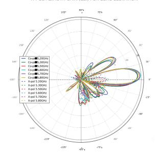
V-POL ELEVATION GAIN (dBi) FOR ZERO AZIMUTH
