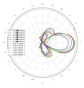
V-POL AZIMUTH GAIN (dBi) FOR ZERO ELEVATION
